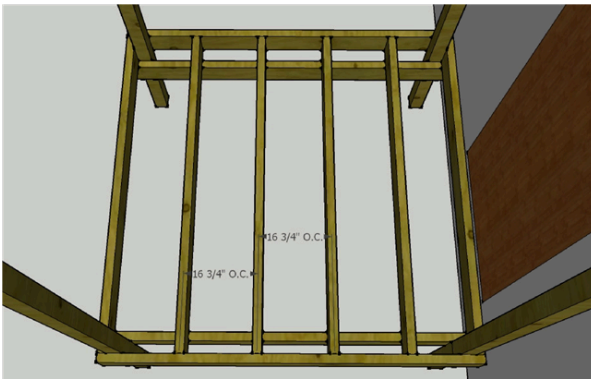
Install common joists
